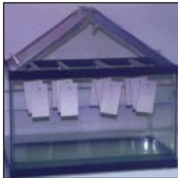
Multiple panels of each test paint are placed in this environmental chamber for six weeks at a high temperature and relative humidity.
